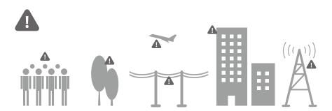
Avoid flying over or near obstacles, crowds, high voltage power lines, trees or bodies of water. DO NOT fly near strong electromagnetic sources such as power lines and base stations as it may affect the onboard compass.
