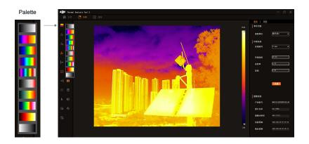
When analyzing the images taken by the Mavic 2 Enterprise Advanced, you can directly drag the chroma bar on the right to adjust the mapping relationship between temperature and color. If you open an image taken by Zenmuse H20T, the isothermal icon ## must be selected first before adjusting the chroma bar.
