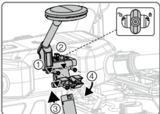
4. Remove the sticker on the GPS kit's cable and then fix the cable onto the aircraft.
