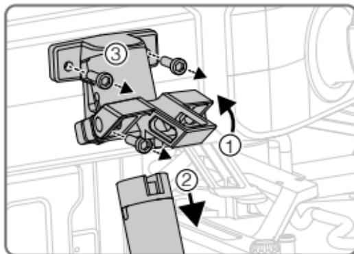
3. Mount the GPS kit with the three screws and then rotate the knob to the lock position. Mount the right landing gear.
