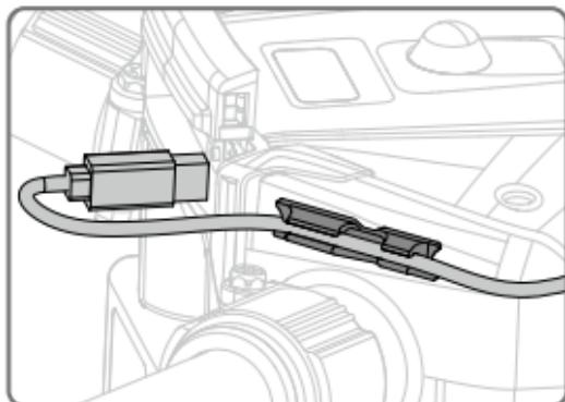
5. Connect the GPS kit's cable to the port as shown.
