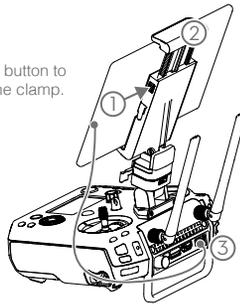
Place your mobile device and adjust the clamp to secure.
