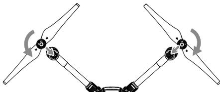
⚠ Check that the propellers are secure before each flight.
