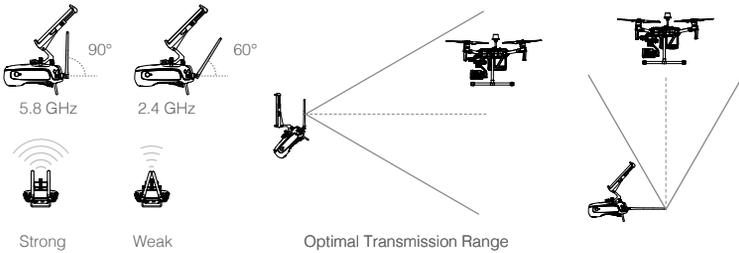
Ensure the aircraft is flying within the optimal transmission zone. To maintain optimal transmission performance, adjust the remote controller and antennas according to the above diagram. The position of the antennas required for optimal transmission range varies in the frequency of 5.8 GHz and 2.4 GHz. Please place the antennas based on the actual operating frequency.
