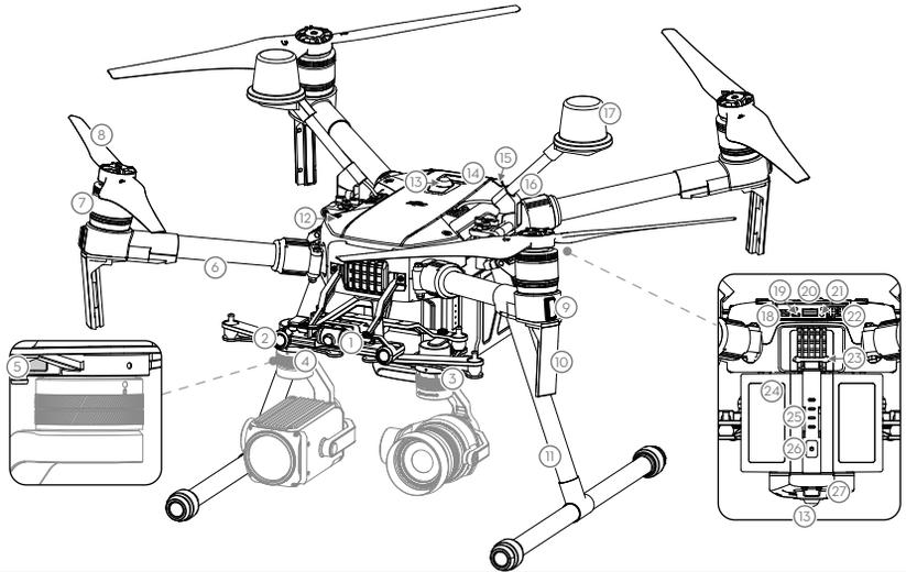
☀ The M200 V2 comes with a single downward gimbal connector. The M210 V2 and M210 RTK V2 each comes with a dual downward gimbal connector. The illustrations in this manual may vary from the actual product.
