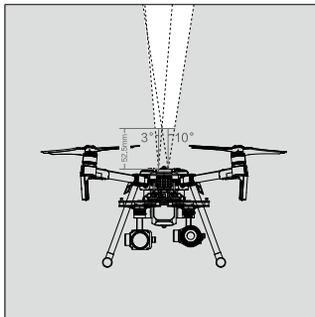
A note on the vision system and the ultrasonic sensor detection range is illustrated below. There may be a  $\pm 2^\circ$  error in the angle of the downward vision system and ultrasonic sensor due to errors in the assembly process. To prevent accidents, please DO NOT attach any payload that might be in the sensors' Do Not Obstruct Zone. If the payload comes into the Do Not Obstruct Zone, it is recommended to turn off the downward vision system in the Pilot app and fly with caution.
