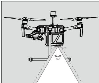
Infrared Sensing System detection range is depicted below.
