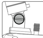
Use a coin or the screwdriver included to adjust the tightness of the tilt axis.
