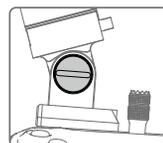
Use a coin or the screwdriver included to adjust the tightness of the tilt axis.
