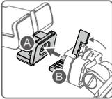
Ensure that Part B is unlocked. Connect Part B to Part A.
