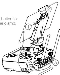
Place your mobile device and adjust the clamp to secure.
