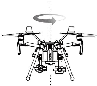
3. Hold the aircraft vertically, with the nose pointing downward, and rotate it 360 degrees around the center axis. Re-calibrate the aircraft if the aircraft status indicators blink red.
