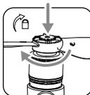
Press the propeller down onto the mounting plate and rotate in the lock direction until secure.
