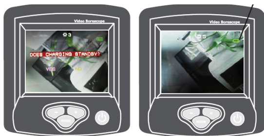
Battery status indication
