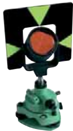
Ref.-No. 481 110-613 Leica-Style Prism Station, tribrach adapter with optical plummet. Accuracy: \pm 2''
